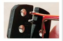
The last step is to insert the connector with the pins into the outer shroud of the female connector. Molded into the shroud there are two small wedges that engage the
