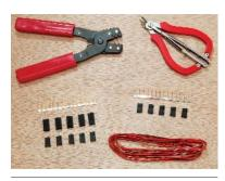
Position the connector in the crimper with the tabs directed into the crimper pocket and the wire exiting on the side with the embossed wire-size markings. Squeeze the handles together firmly. With a little care, you can feel when the crimper does its job and locks the joint. Remove the connector, and give the wire a firm tug.
